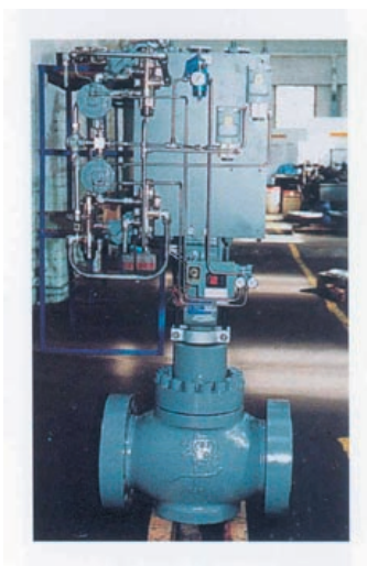
8", 1500 ANSI Compressor recycle valve retrofitted with DRAG trim
