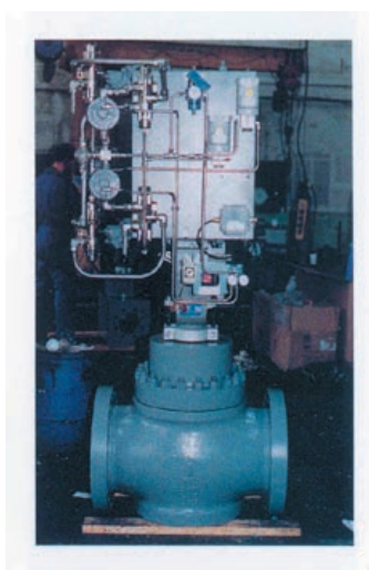
12", 600 ANSI Compressor recycle valve retrofitted with DRAG trim
