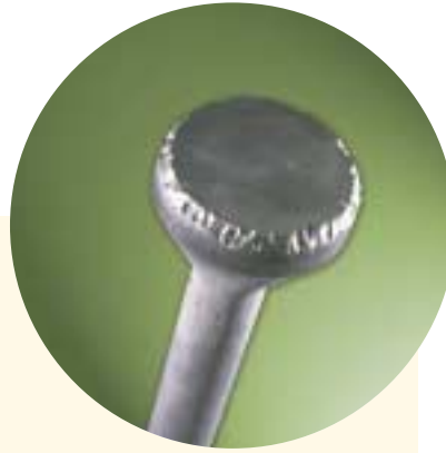
Typical valve trim damage due to cavitation/erosion/vibration in severe service applications.
