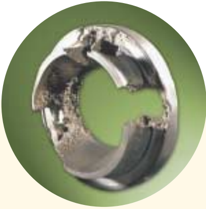
Typical valve trim damage due to cavitation/erosion/vibration in severe service applications.
