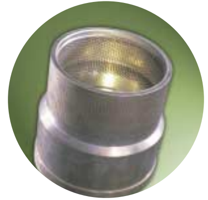
Typical valve trim damage due to cavitation/erosion/vibration in severe service applications.
