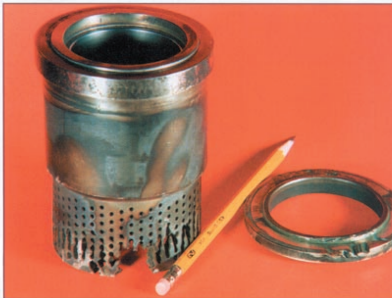
Fig. 1: Single-stage, pressure-reducing valve trim severely damaged by high-velocity gas flow containing corrosion products.
