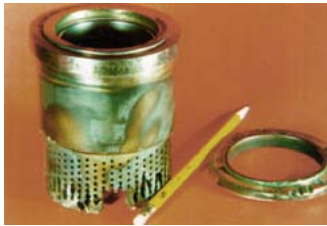
Figure 6: The damaged single-stage trim in a gas pressure letdown valve.
