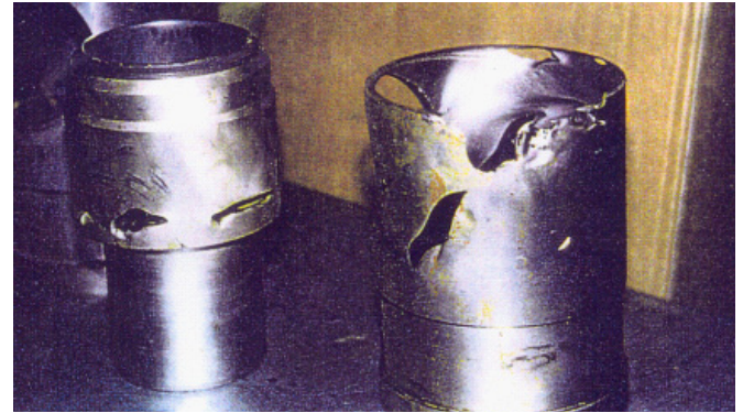
Competitor's single stage trim after less than a week
